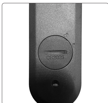
Remote battery replacement
